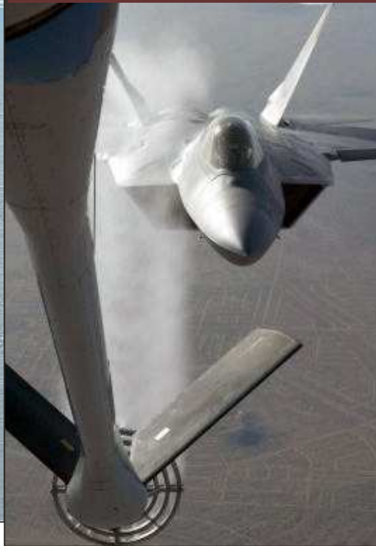
A modified KC-135 sprays water on an F-22 during icing tests at Edwards AFB
